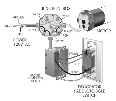
CAUTION: Before proceeding with the line voltage wiring instructions, the up and down limits of each motor should be set using the SOMFY tester cable (Cat. No. 6020086). Refer to the limit switch instructions packaged with each SOMFY motor for more information.
